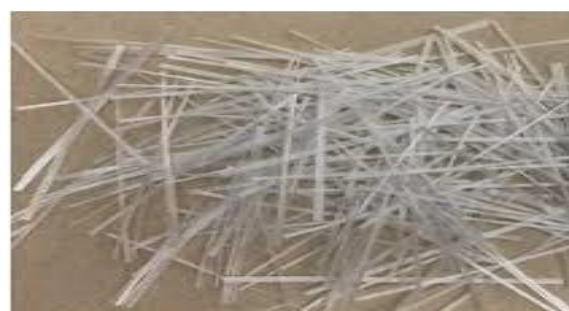
Figure 2: Electrical Waste Glass Fibre
